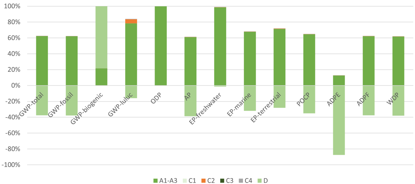
Relative contribution of considered life cycle stages - Welsch profiles made of hot-rolled steel
