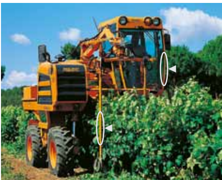
Cab section as well as axle for the guide tracks of grape harvesting machines.
