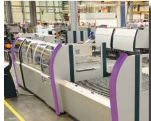
Covered bent columns shown here guarantee the machine operator's safety.
